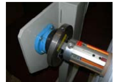
Securing pneumatic axe in clasp bearings
